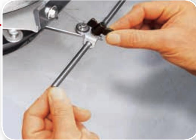
Easy and simple adjustment on graduated scales with 50 positions. If necessary, the system enables to feed the two discs with different quantities.
