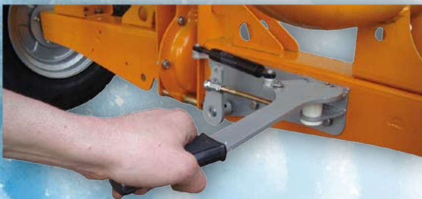
◀ Engagement/disengagement lever of the spreading disc Engagement et desengagement de la rotation du disque
